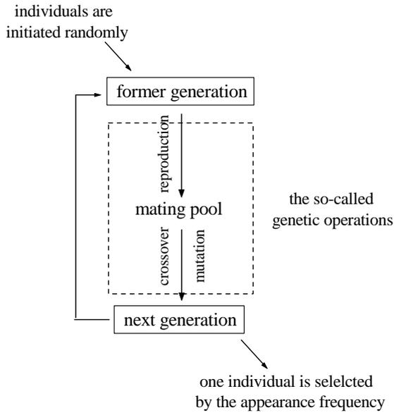
**Fig. 6. Schematic illustration for the genetic algorithm.**
