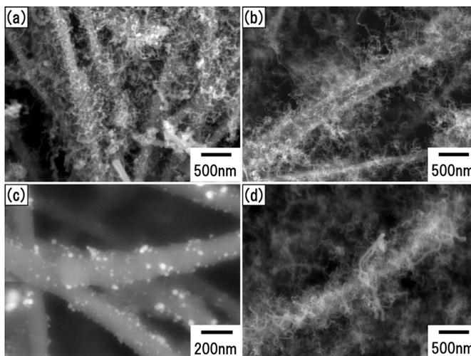
Fig.1. SEM images of CNTs grown on CNFs by Co-DBA (a) and Ni-SDS (b) treatment, (c) Co catalyst adhered on CNFs by chemical precipitation process, (d) CNTs grown from (c).
