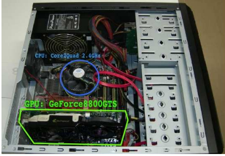
Fig. 4. A high-speed POC/RIPOC calculation system by GPU
