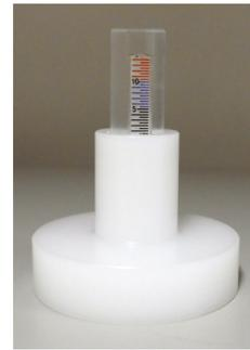
**Fig. 1.** Instrument to measure the depth of the surface imprint
