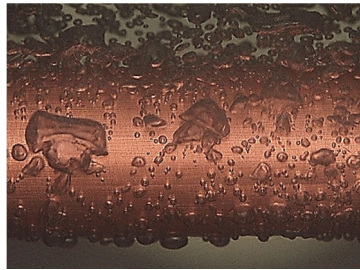
(d) R1234ze(Z) at 20 °C ( p_{\text{red}} = 0.04 ) and 20 kWm -2 , \alpha = 2.46 kWm -2 K -1
