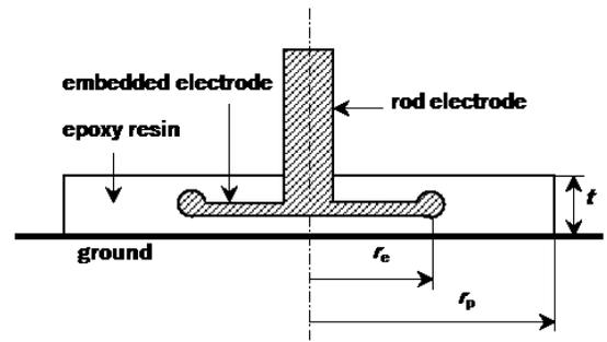
**Figure 1.** A design model of composite insulation system with embedded electrode.  $r_p$  is the radius of the disc-type epoxy resin plate,  $r_e$  is the radius of the embedded electrode and  $t$  is the thickness of the epoxy resin plate.
