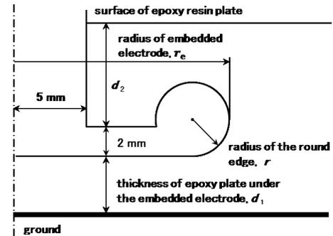
**Figure 2.** An enlarged diagram of the region around the edge of the embedded electrode.
